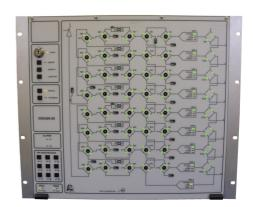
The DDA286 is a family of units and modules for switching controllers (including LNA/LNB controllers) and switching systems where a network port is desirable. A modular construction allows support for virtually any configuration, and non-standard features can be incorporated on request.
