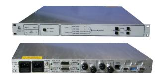
The DDA291 is intended for beacon monitoring applications. It is a fully integrated unit, incorporating the beacon receiver, mains supplies, LNB power supplies and input switching in one compact 1U high rack mount unit.
