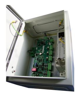
The DDA293 is intended for the smaller waveguide switch control applications where rack mounting (and a local display) is inappropriate, and can be provided in a variety of configurations.
