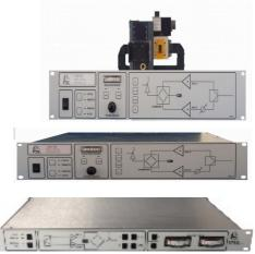
The DDA78 family manages the phase combining of a pair of HPAs using CRCA combiners from manufacturers including Luso, Flann, Mitec and Comdev. It manages the various RF switching options. The package includes the phase adjuster and RF splitter.
